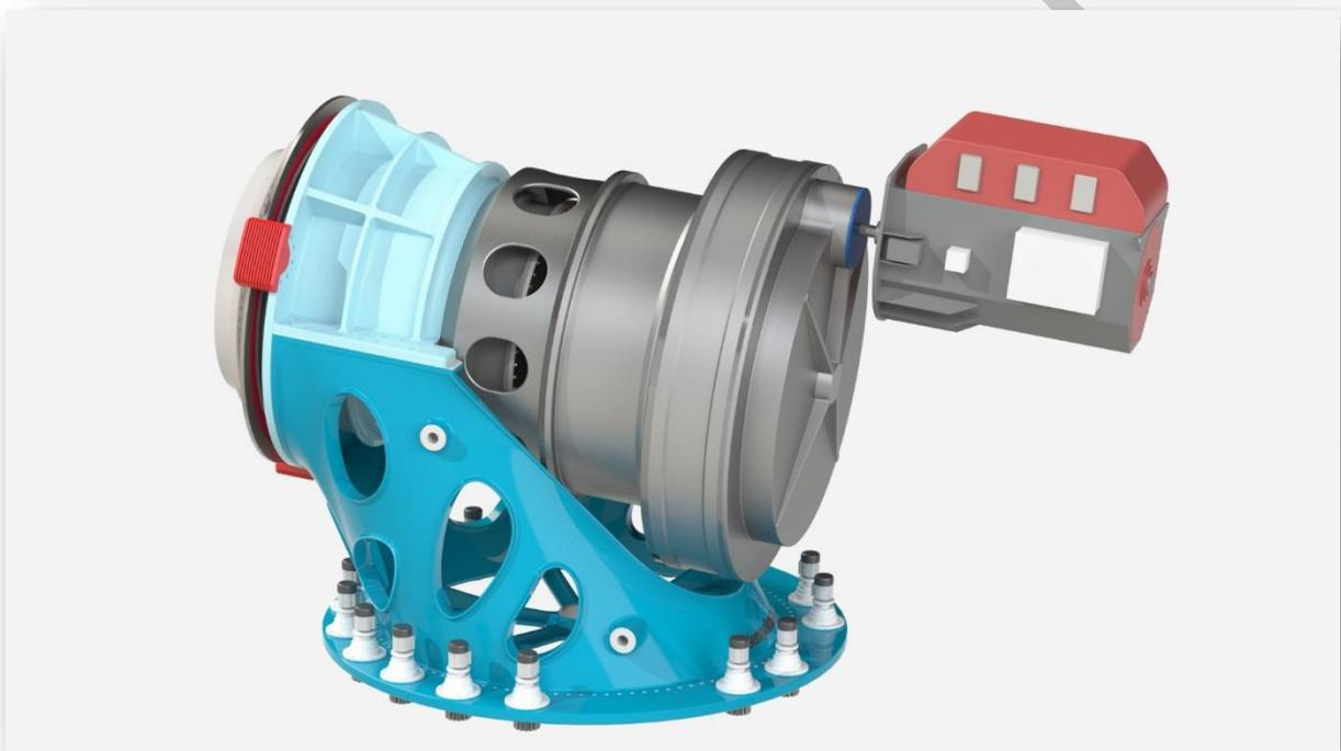
The MergedGear gearbox can be divided into two parts: the first part is the innovative stepped planetary gearbox, the second a parallel step connected to the generator.
